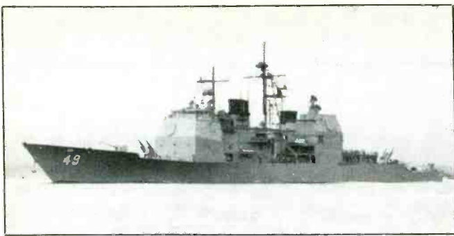
Jerry Cody, WA took this fine photo of the USS Vincennes, CG-49. The ship, commissioned 6 July 1985, is 567 feet long and 55 feet wide. Weighing in at 9400 tons, it is one of the larger of the ships comprising the 1987 fleet. It employs an AEGIS missile system to defend against enemy missiles. Note all the antennas including some COMSAT dishes. Callsign: NVIN.
