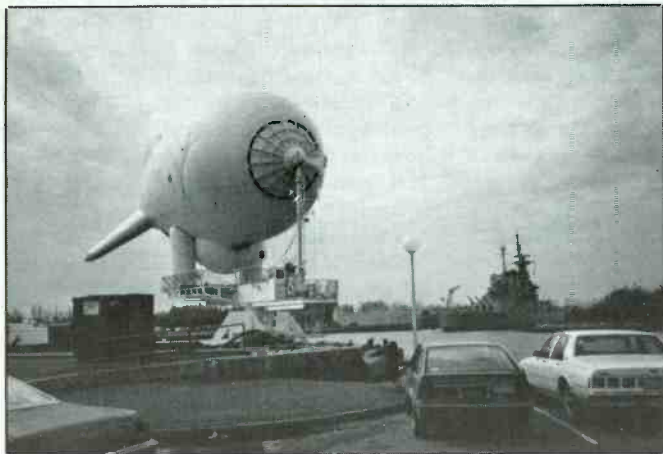
STARS means Small Tethered Aerostat Relocatable System. Radar antennas located in the pod beneath the aerostat (an unmanned blimp kept on a leash tied to a ship) can get a good look at distant ships and aircraft once the aerostat is sent aloft. Operators located on the vessel radio the vectors to pursuit aircraft and ships. It's being considered for use in hunting drug smugglers. This one, on the vessel American Sentry, was spotted while moored in the Washington, DC area. Note the battleship in the background. (Photo courtesy Alice Brannigan.)
